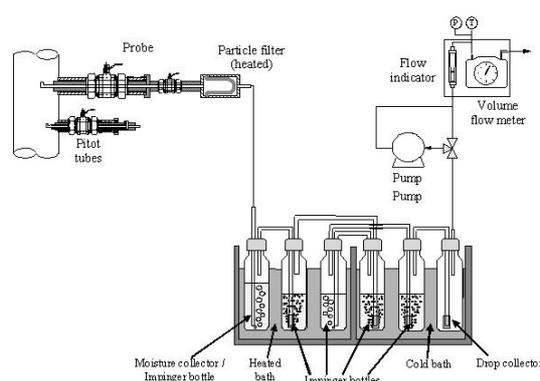
**Figure 1.** The TMS sampling set-up: atmospheric and isokinetic sampling train for tar and particles with removable probe and Pitot tubes for flow measurement. Set-up Guideline +40, +40F, -20F, +40F, -20F, -20F
