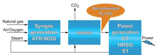
Power production with CO<sub>2</sub> capture by SEWGS. Power is generated by gas turbines (GT) and steam turbines (ST), heat is recovered for steam generation (HRSG). Steam is needed for autothermal reforming and water gas shift (ATR/WGS), and for CO<sub>2</sub> removal by SEWGS.
