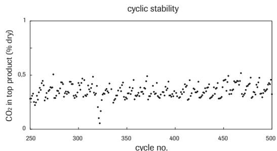
Long term stability test of new K-MG30 sorbent
