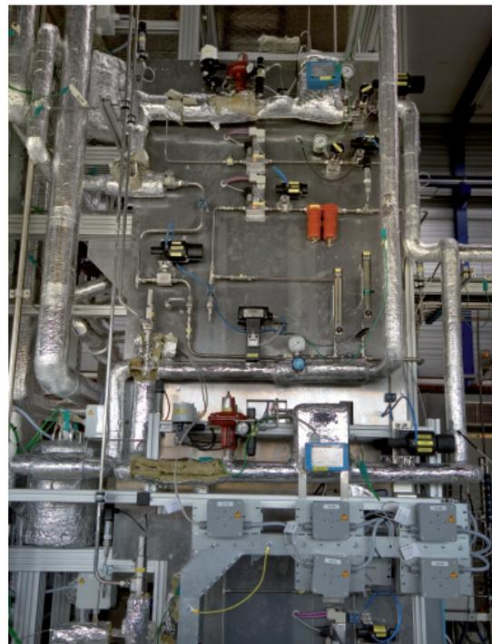
Feed section for supplying, mixing and heating gases and steam
