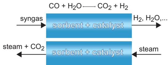
SEWGS principle: (upper) adsorption and reaction at high pressure (lower) desorption at low pressure
