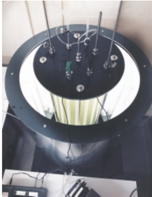
The ECN bench scale photobioreactor
