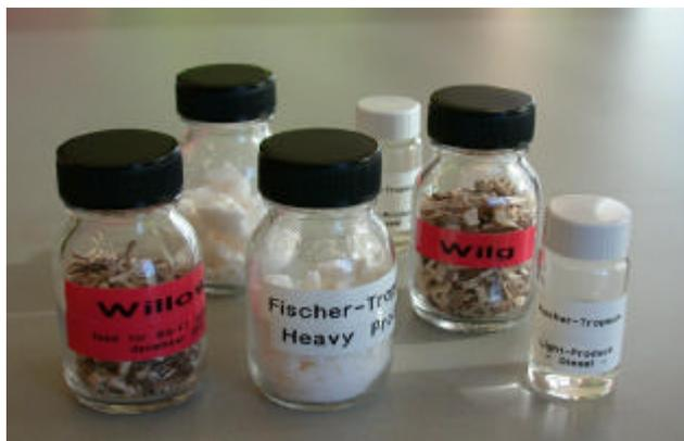
Figure 7. Pictures of the willow used for the integrated test, Fischer-Tropsch wax, and the light product (viz. 'green diesel').
