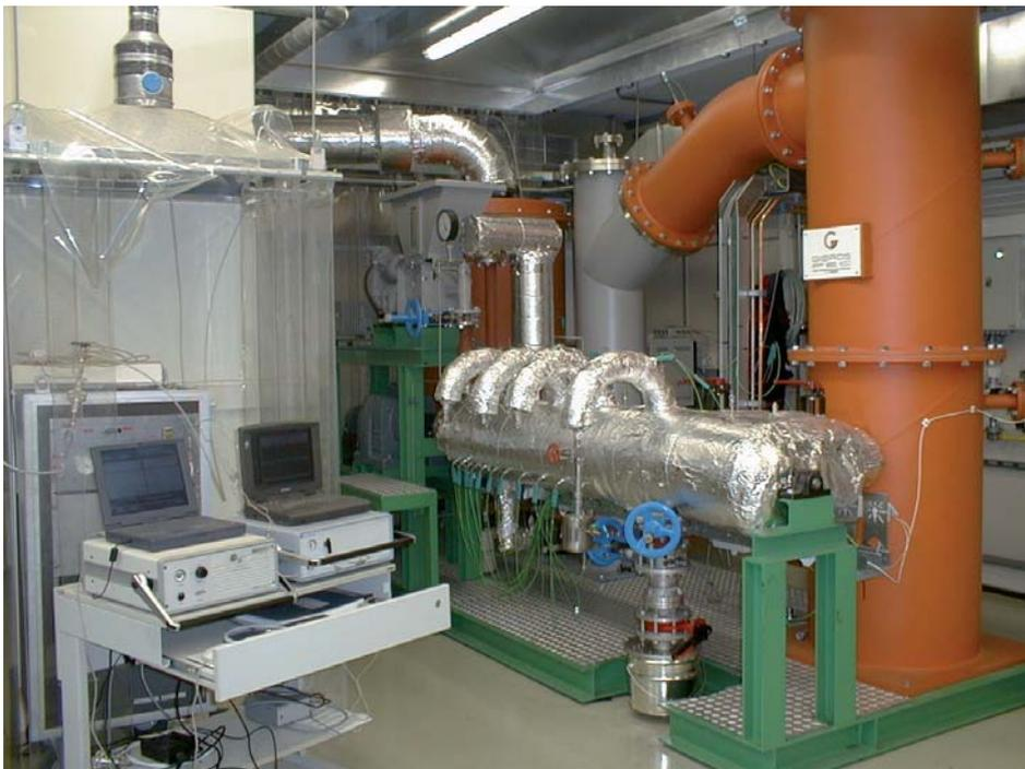
*ECN Bench-scale reactor for producing batches of up to 5 kg biochar*
