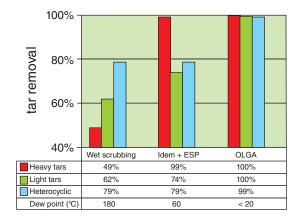
The most important result is that the tar dew-point of the gas can be decreased to well below 20°C. This means that the gas is applicable without risk of tar condensation and fouling
