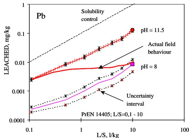
Figure 9 Evaluation of external influences on release from MSWI bottom ash for Pb.
