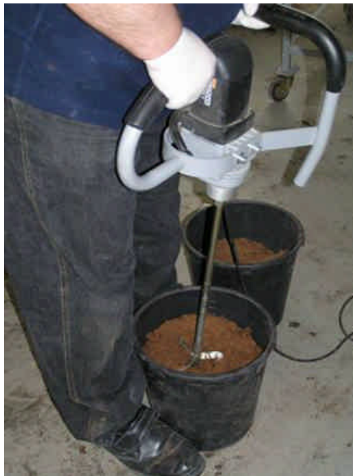
Figure 3: Mixing of control substrate and digestate
