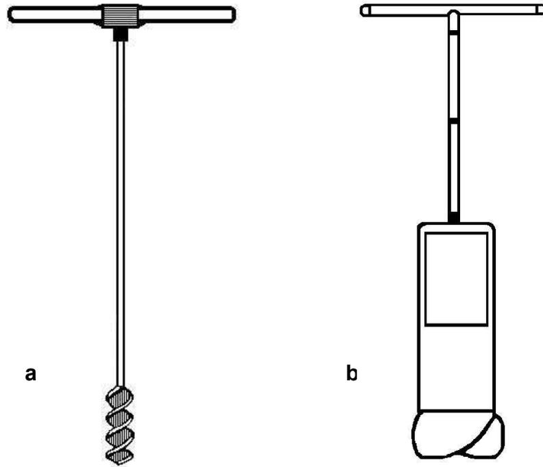
Figure B.1 — Sampling augers (a) Screw auger; (b) Bucket auger
