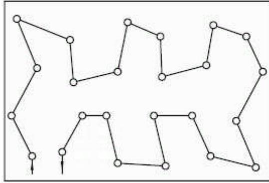
Figure A.2 — Zigzag traverse sampling pattern [ISO 10381-1:2002]
