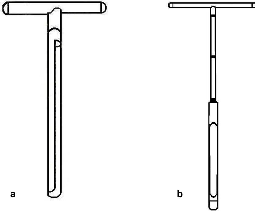
Figure B.2 — Push samplers (a) Trier; (b) Tube sampler
