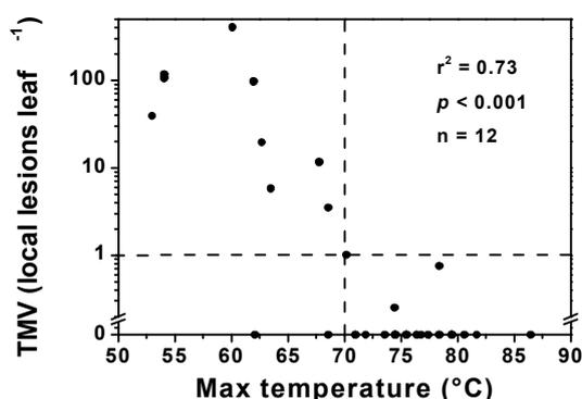
**Figure 1.** Survival of *Tobacco Mosaic Virus* (TMV) correlated with the maximum temperature obtained during 2-4 week sanitation in four large scale compost facilities (Christensen *et al.* 2001)
