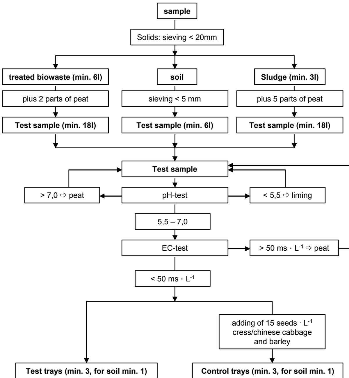
Fig. 2: Flow chart of the testing procedure
