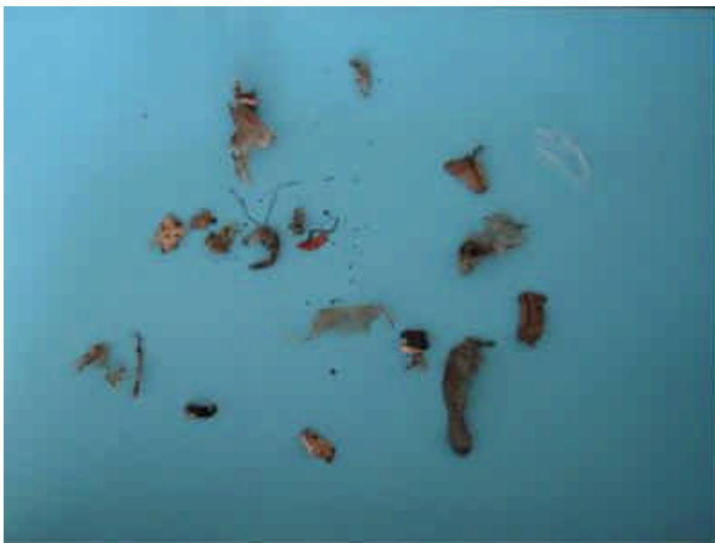
Figure 1 Selected plastics on a blue sheet, note the rumpling and discolouration
