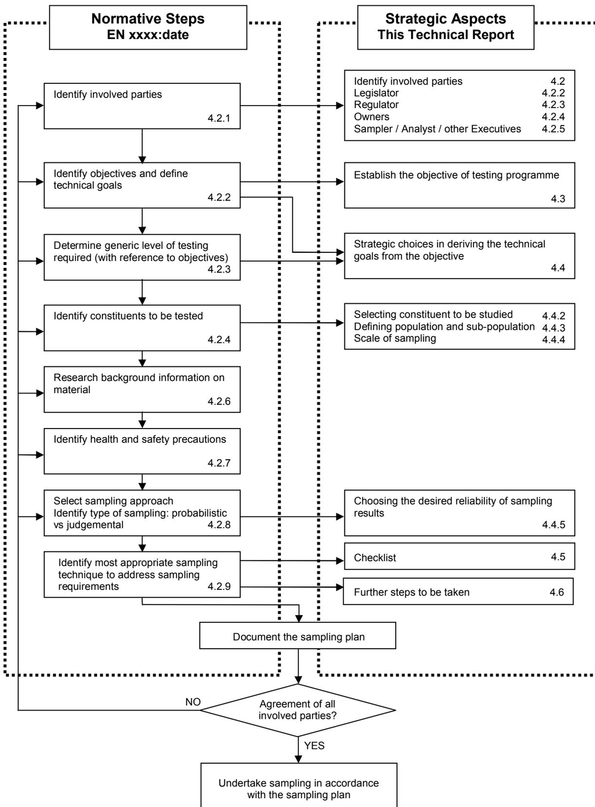
Figure 1 — The process of defining the sampling plan
