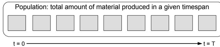
**Figure 3 — Continuous production of a homogeneous material**
