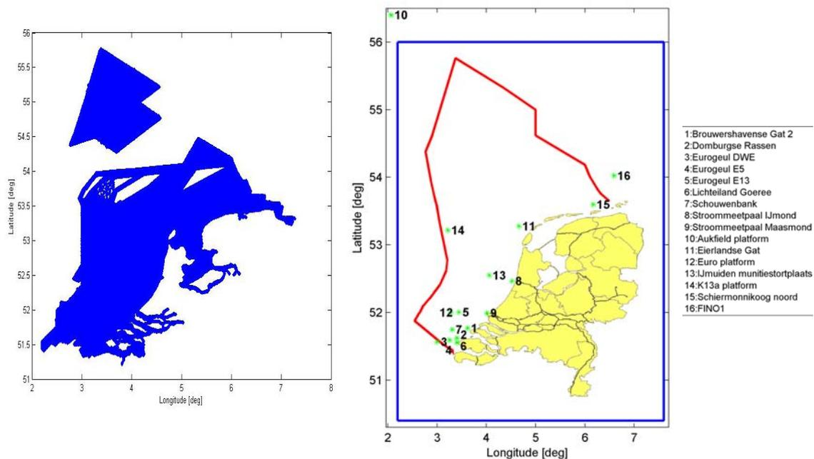
Figure 2 Locations where sea depth (left) and wave data (right) are known. In order to estimate sea surface roughness these data are interpolated to the location of interest by inverse distance weighting
