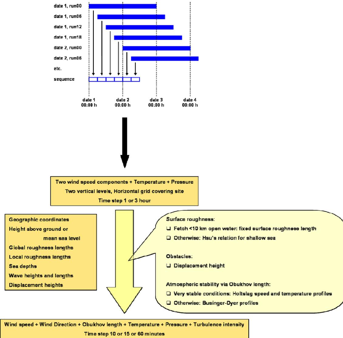
Figure 1 Construction of a long-term time series of wind data and vertical interpolation of these data
