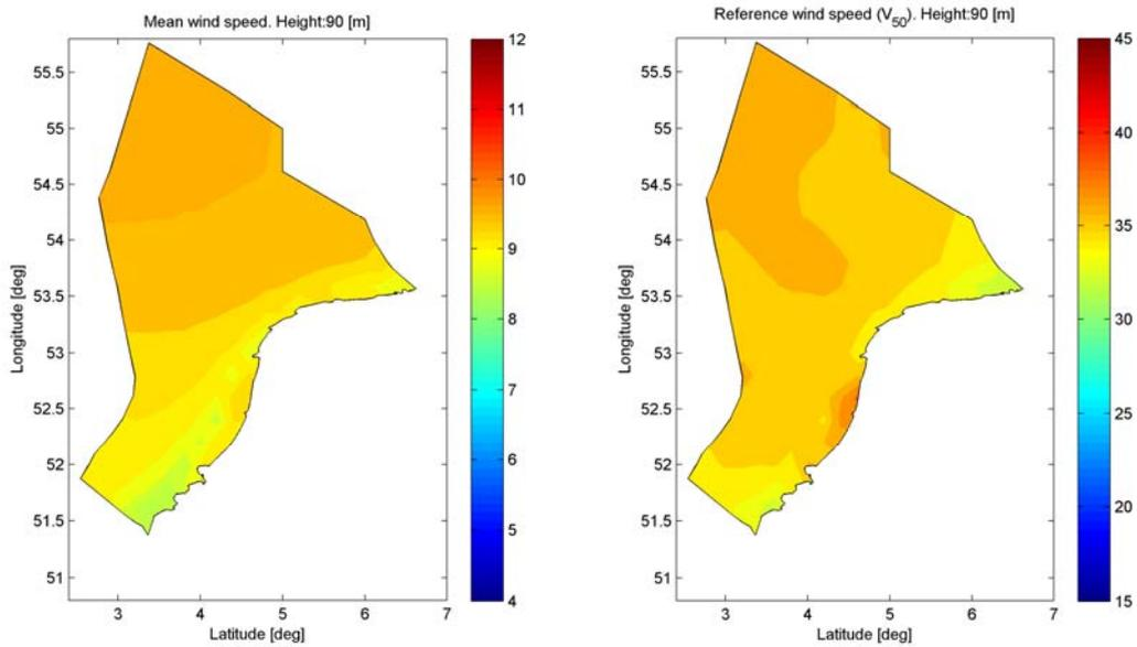
Figure 4 Mean wind speed (left) and reference wind speed (right) at a height of 90 meter in the Netherlands' Exclusive Economic Zone
