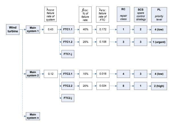
Figure 5-2: Breakdown of the turbine and grouping of maintenance activities for the O&M *Calculator.*
