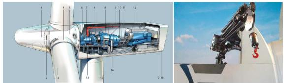
Figure 2-3: Examples of internal cranes in the Siemens 3.6 (left) and Repower 5M (right) turbines
