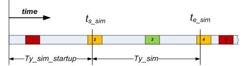
Figure 7-1: Simulation period and possible repairs due to simulation period selection; ts\_sim and te\_sim are the start time and the end time of a certain simulation period (i.e. the next 1, 2, ..., 5 years), and Ty\_sim\_startup is the start-up period
