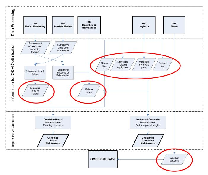
Figure 9-2: Interfaces between the OMCE-BB's and OMCE-Calculator
