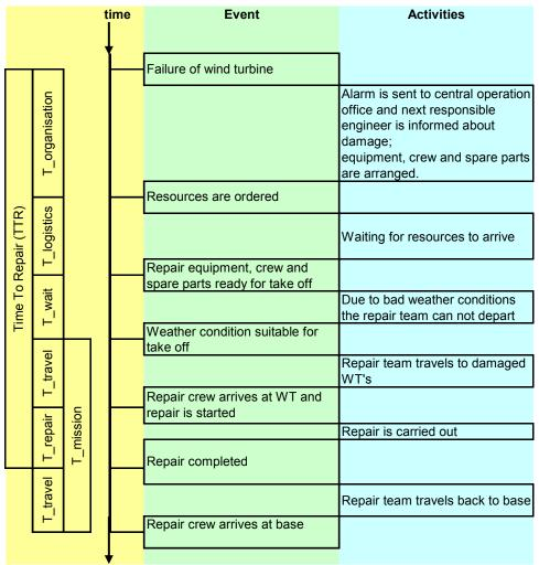
Figure 2-9: Maintenance process for unplanned corrective maintenance
