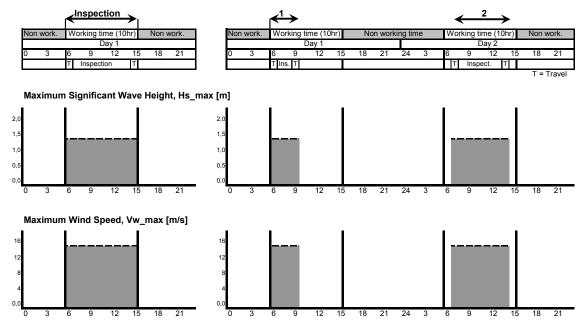
Figure 5-5: "Inspection" of 8 hrs with 1 hour travelling to and from the turbine - continuous action (left), or - split up (right)
