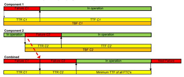
Figure B.3: Illustration of two component failures and the delay in repair of component 2
