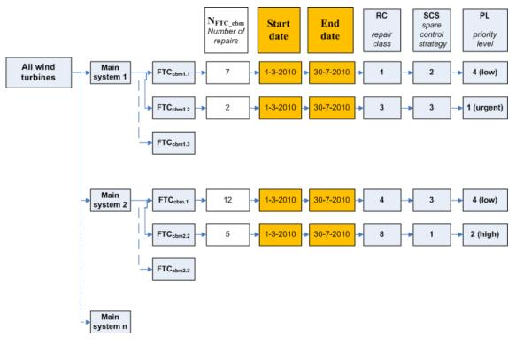
Figure 5-8: Definition of FTC's for condition based maintenance (subscript "cbm" = condition based maintenance)
