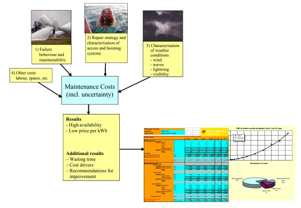
Figure A-1: Schematic representation of the ECN O&M Tool for determining the O&M costs and downtime of an offshore wind farm.
