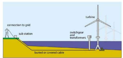
Figure 2-1: Typical lay-out of an offshore wind farm [Ref. 9]
