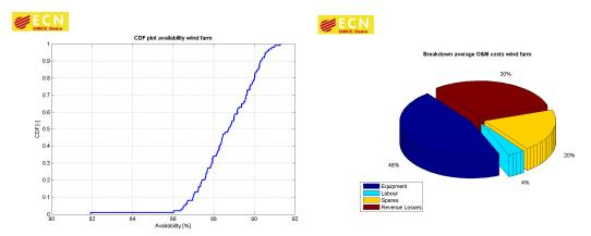
Figure 8-8: OMCE-Calculator post-processor plot output, CDF availability wind farm (left) and breakdown of O&M costs wind farm (right)
