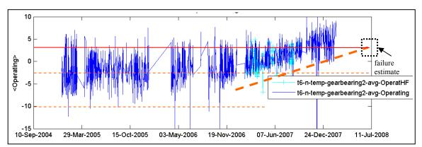
Figure 15-1: *Example of a visualisation from de-trended SCADA statistical data; slow increase of the bearing temperature indicating wear*
