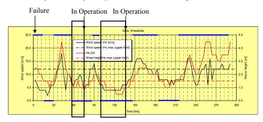
Figure B.4: Example of determination of waiting time for a maintenance action that can be carried out if  $H_s \le 1.5$  m and  $V_w \le 12$  m/s and the duration is 20 hrs or 40 hrs.
