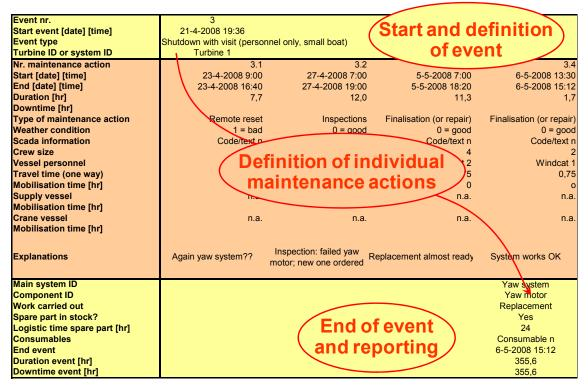
Figure 11-3: Report of an alarm leading to an immediate shutdown which requires three on site visits after a remote reset has been tried first; the downtime is equal to the total duration of the event
