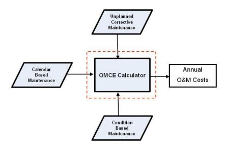
Figure 4-1: OMCE Calculator to model 3 types of maintenance and estimate O&M aspects
