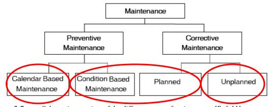
Figure 2-7: Schematic overview of the different types of maintenance [Ref. 11]
