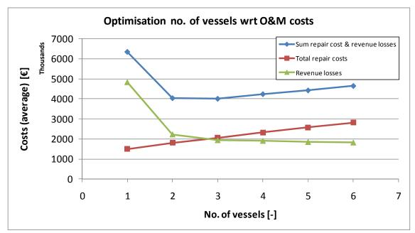
be related to the increase in repair costs and the decrease in revenue losses. The number of available vessels with respect to repair costs and revenue losses is now plotted in Figure 8-11.
