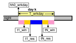
After day k has been processed and the work is not completed yet, the process is continued by finding the next day with a suitable weather window, and this search starts at day k+1. When the next suitable weather window is not found on the next day (day k+1) but on on day k+n (with n>1) the waiting time due to the weather conditions is raised with (n-1)\*24hours.
