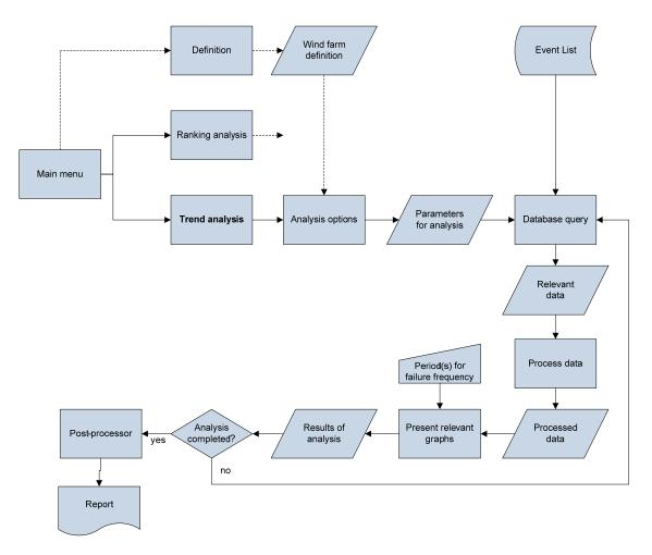
Figure 12-2 Flowchart for performing trend analysis of the maintenance data using the building block 'Operation & Maintenance'.
