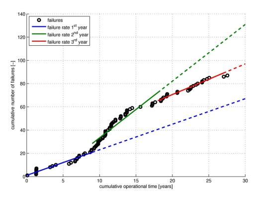
Figure 12-5 *Example of a CUSUM-plot used for visualizing trends in failure behaviour.*
