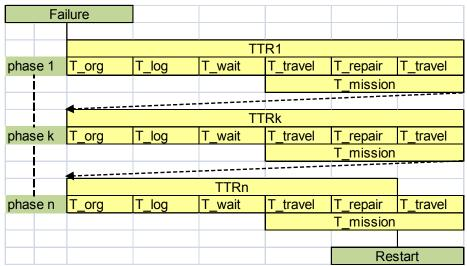
Figure 5-3: Sequence of maintenance phases
