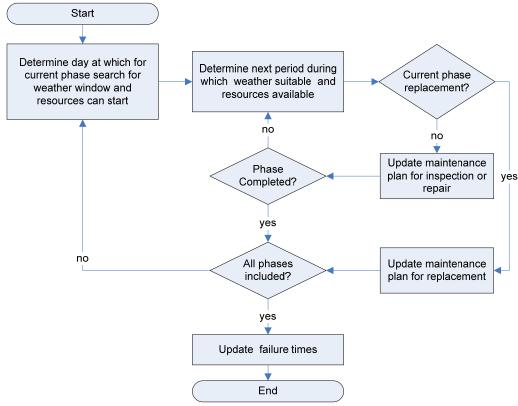
Figure 6-3: Flowchart describing the general approach for processing corrective maintenance.
