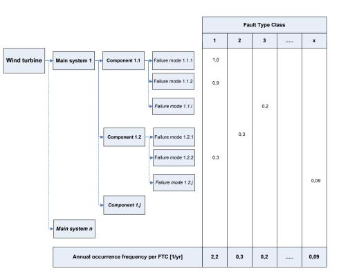
Figure A-4: Process of grouping small and severe failures into manageable set of FTC's
