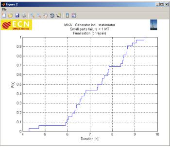
Figure 13-4 *Example of the output of the RPC characterisation of the Building Block* 'Logistics'. Here the CDF of the duration of a small repair on the generator is shown.
