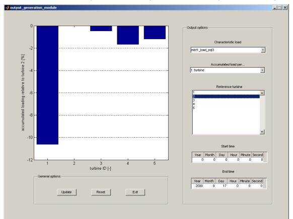
Figure 14-5 *Example of the output generation model of the Flight Leader software, where the relative (to turbine 3) load accumulation of all turbines is displayed.*
