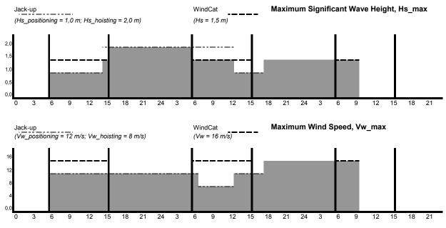
Figure 5-6: "Replacement" of gearbox; maximum allowable weather conditions indicated as grev areas
