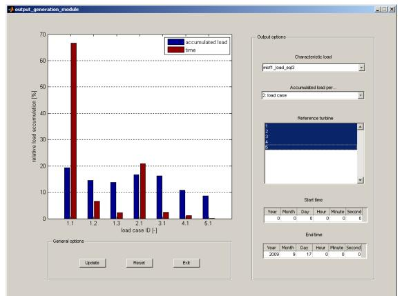
Figure 14-6 *Example of the output generation model of the Flight Leader software, where the contribution of each load case to the total load accumulation is shown.*
