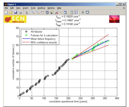
Figure 12-11 Example of the output of the trend analysis of OMCE Building Block 'Operation & Maintenance'.
