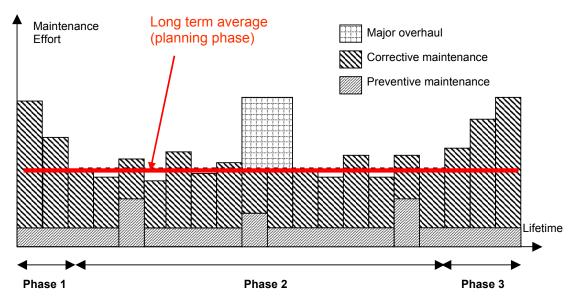
Figure 2-8: Schematic overview of the maintenance effort over the lifetime of a turbine. In reality, none of the lines is constant; the actual maintenance effort will vary from year to year.
