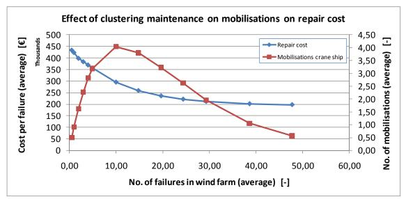
Figure 8-13: Effect of clustering maintenance on number mobilisations and repair cost
