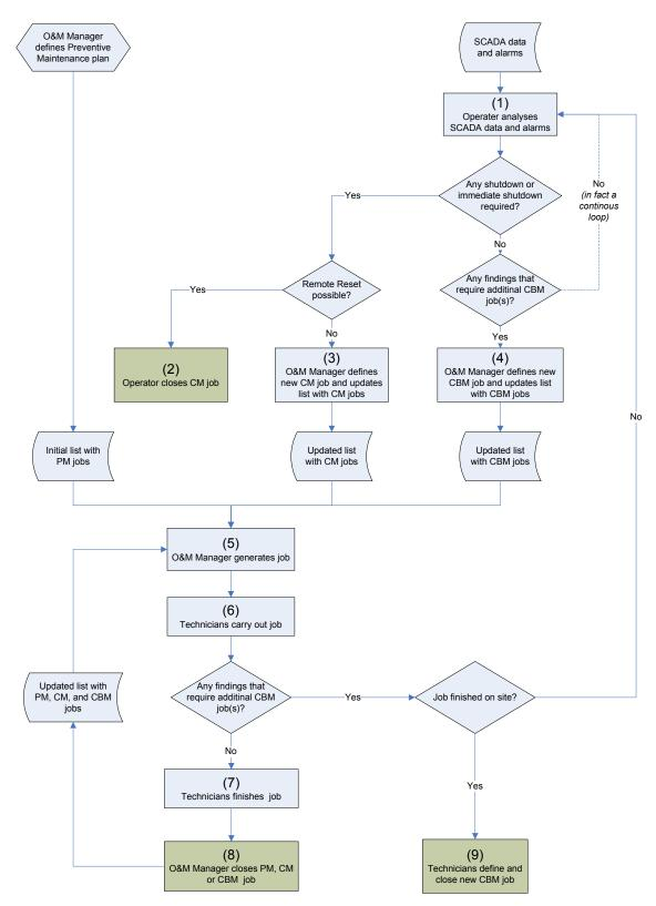
Figure 11-5: *Example of a workflow for maintaining an offshore wind farm which ensures the connection between the an event and the individual maintenance actions*
