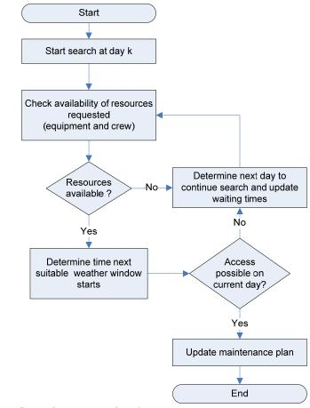
Figure 6-4: Process flow of insertion of replacement
