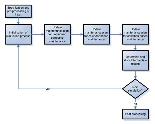
Figure 6-2: Basic schematic overview of the modelling process of the different types of maintenance.
