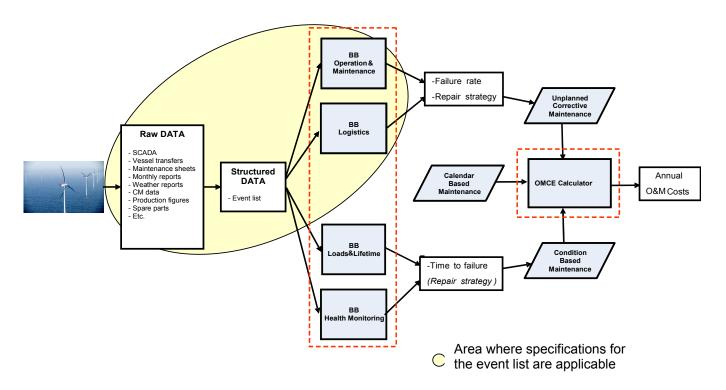
Figure 3-1: OMCE concept including the process of structuring the raw data into an event list
