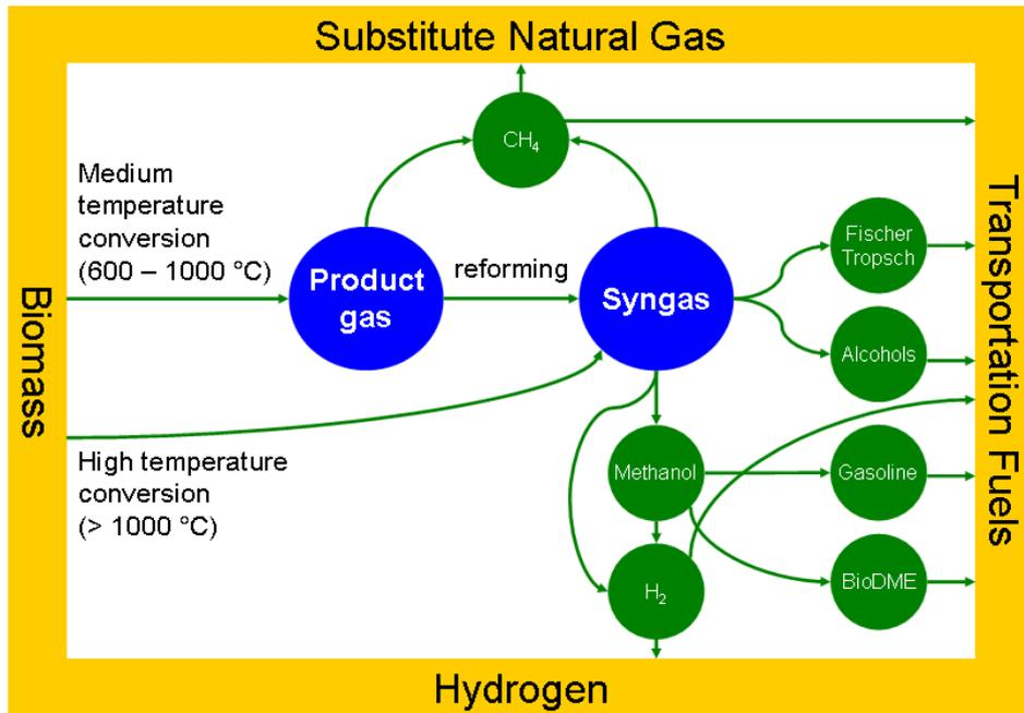
Figure 4.2 Products from the gasification of biomass (Smit, 2009)
