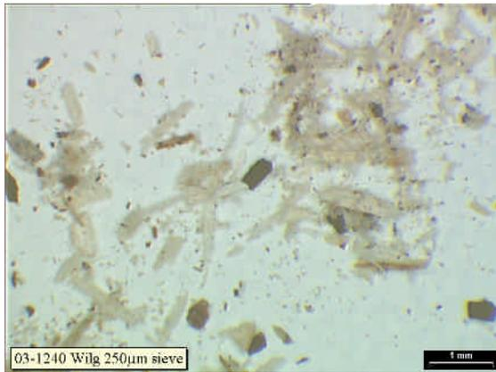
A: Fresh willow milled in the cutting mill with bottom sieve of 250  $\mu\text{m}$
