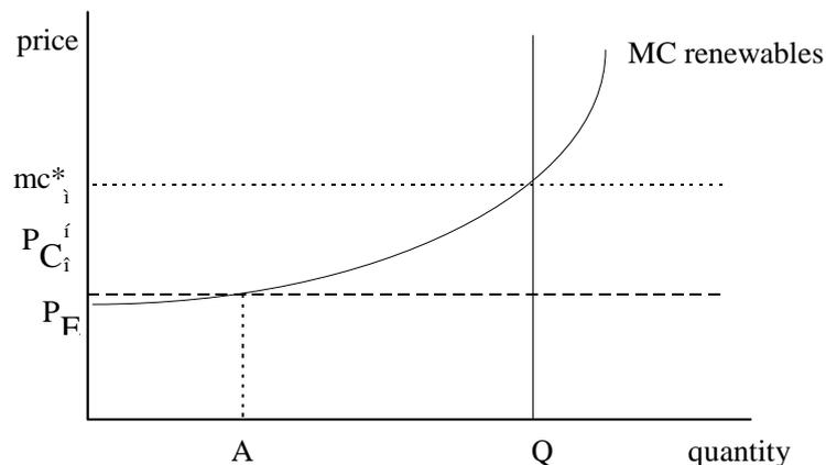
Figure 2.1 *Marginal production cost curve of electricity from renewable energy sources [MC]*
