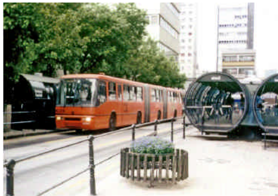
Figure 5.2 BRT system of Curitiba with modernistic 'tubed' stations and bi-articulated busses Source: Wright, 2005.
