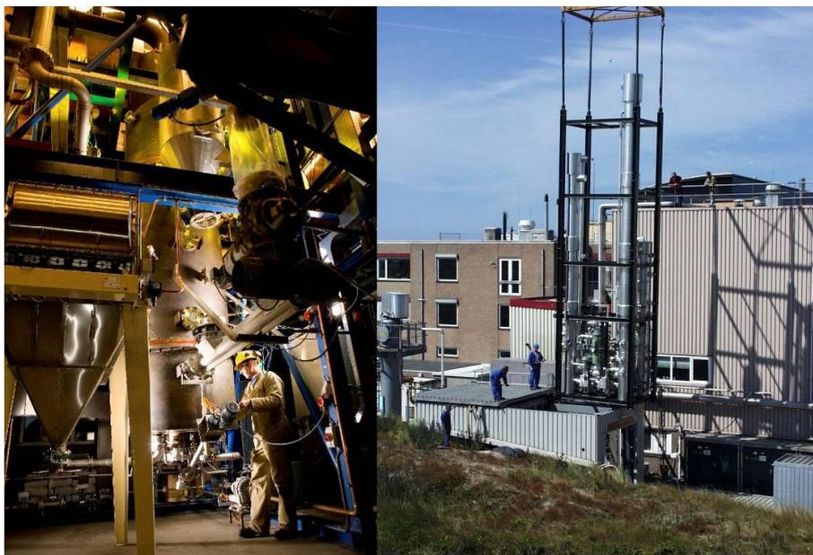
Figure 8: Pilot-scale MILENA gasifier (left) and installation of the OLGA pilot-scale gas cleaning (right).
