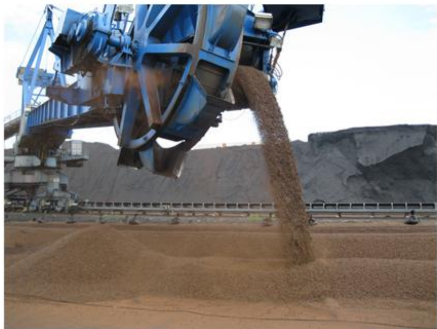
Stacker/Reclaimer in operation
