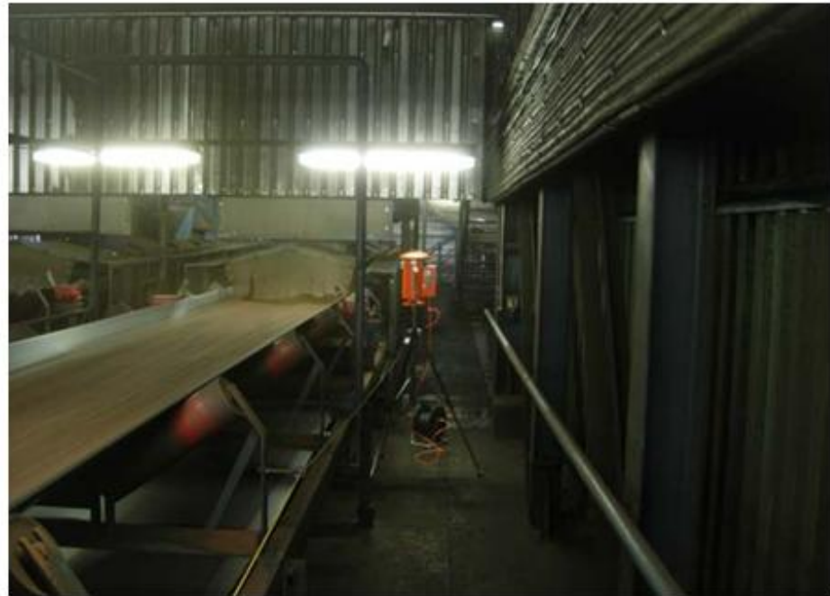
Airborne dust measurements within at a.) conveyer belt and b) transfer point at tower
