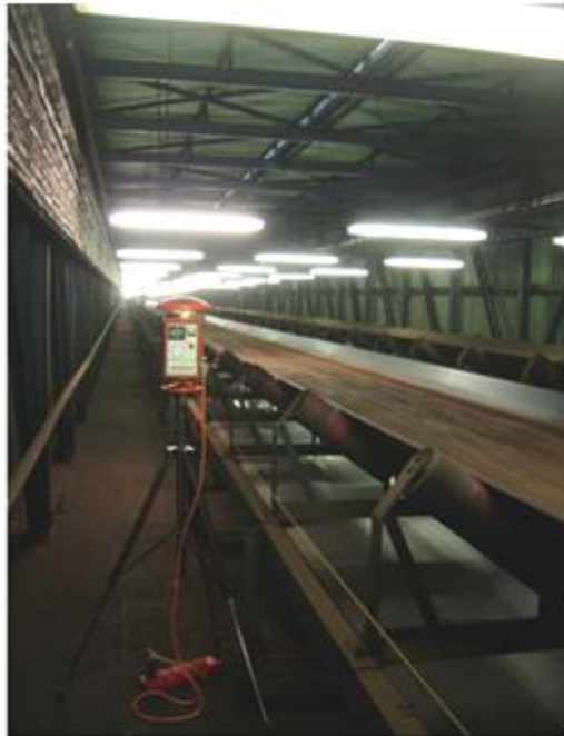
Airborne dust measurements within at a.) conveyer belt and b) transfer point at tower
