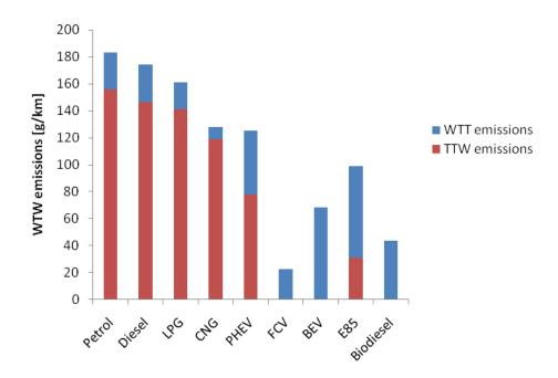
Figure 2.1 WTW-emissions of different vehicle-fuel combinations Note: Excluding emissions from land use changes and non-CO<sub>2</sub> greenhouse gases. Numbers reflect values for vehicles equivalent to a medium-sized, average-efficiency <u>new</u> vehicle.
