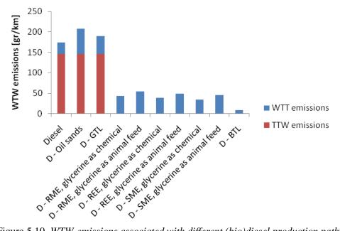
Figure 5.10 *WTW-emissions associated with different (bio)diesel production pathway* Source: JRC et al., 2007.
