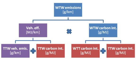
Figure A.1 Calculation of vehicle WTW-emissions
