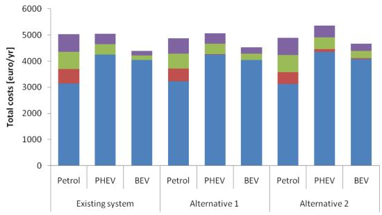
Figure 5.12 User costs of BEVs and PHEVs in the three fiscal systems in 2010 Note: Numbers are values for vehicles equivalent to a medium-sized, average-efficiency <u>new</u> vehicle, 15000 km/yr
