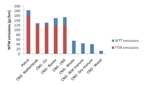
Figure 5.4 *WTW-emissions associated with different CNG production pathway* Source: JRC et al., 2007.
