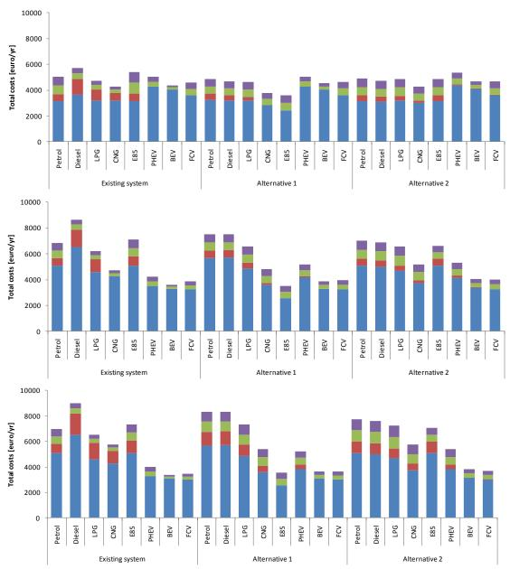
Figure 6.4 Vehicle costs from user perspective of conventional and alternative fuels in the three fiscal systems in 2010 (above), 2020 (middle) and 2030 (below) Note: Numbers are values for vehicles equivalent to a medium-sized, average-efficiency <u>new</u> vehicle, 15000 km/yr.
