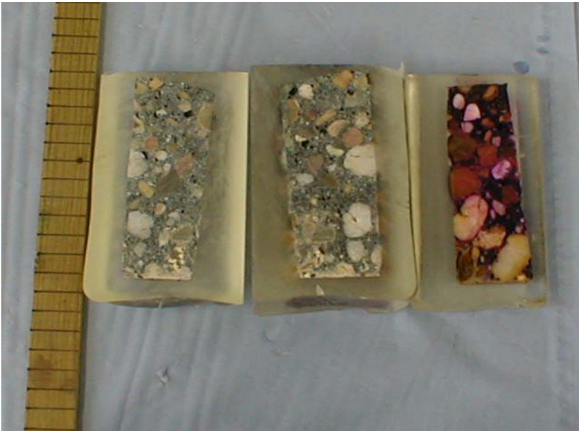
Figure 2.7 *Phenolphthalein dye colouring of the core from the cooling channel of the HFR*
