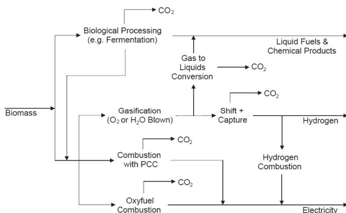
Figure 4.1 Routes to biomass with CO<sub>2</sub> capture and storage (Rhodes and Keith, 2003)
