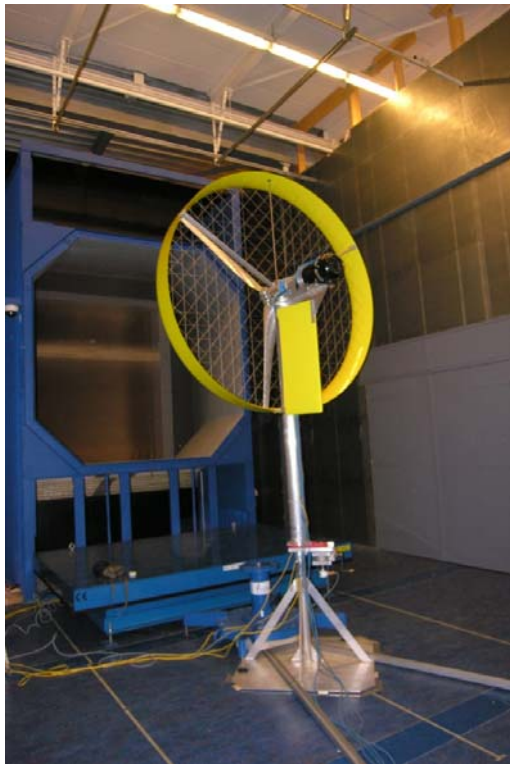
Figure 5: Measurement set-up with test model positioned in front of the wind tunnel nozzle.
