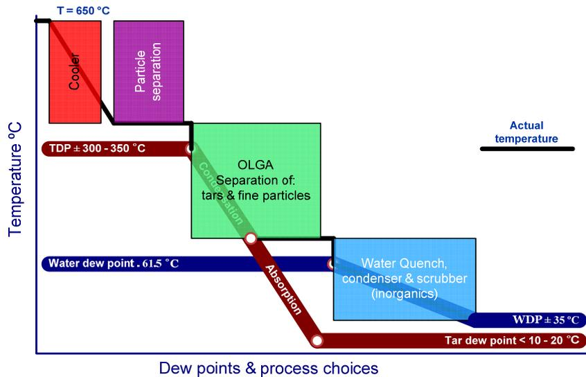
Figure 3.20 *LT-CFB 100 kW<sub>th</sub> basic OLGA working principle*
