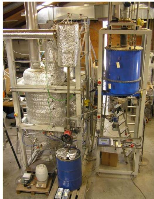
Figure 2.14 100 kW<sub>th</sub> LT-CFB gasifier
