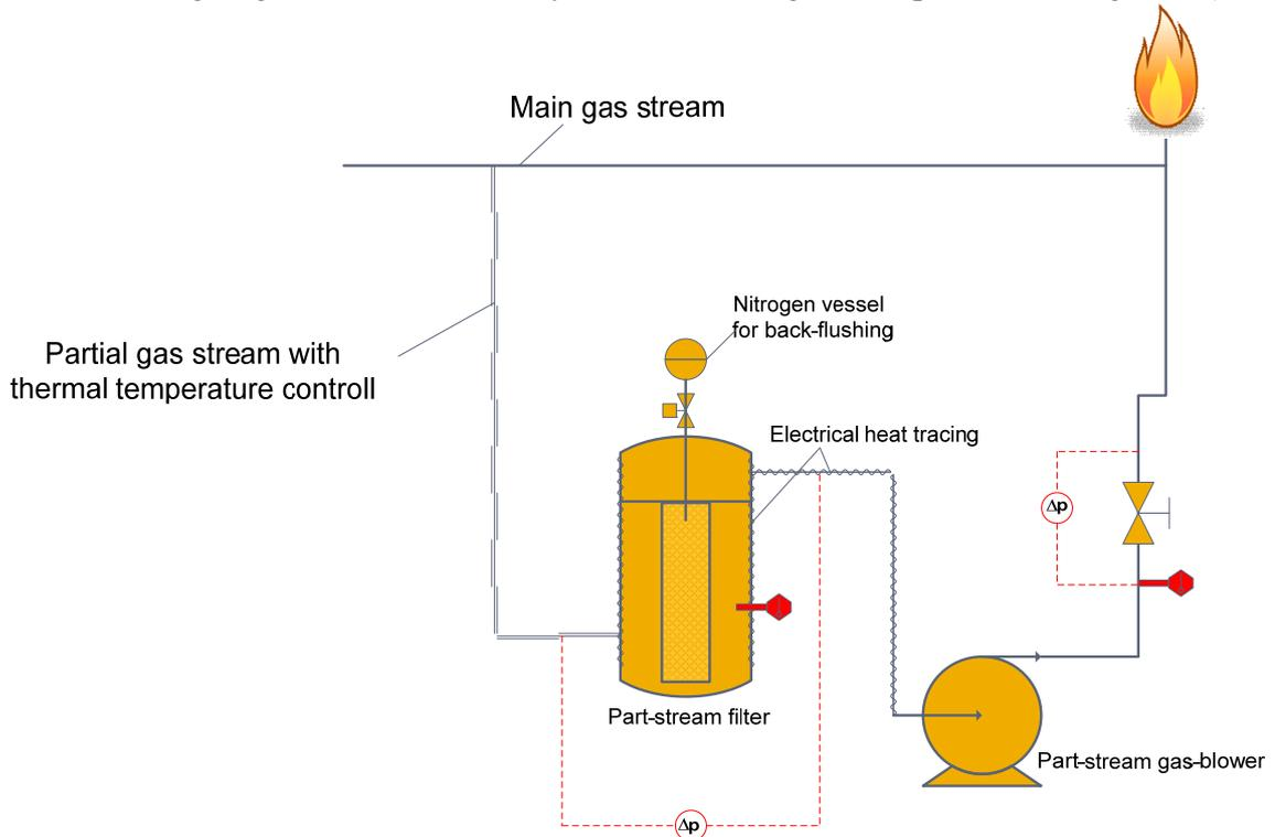
Figure 4.5 Diagram of the filtration set-up
