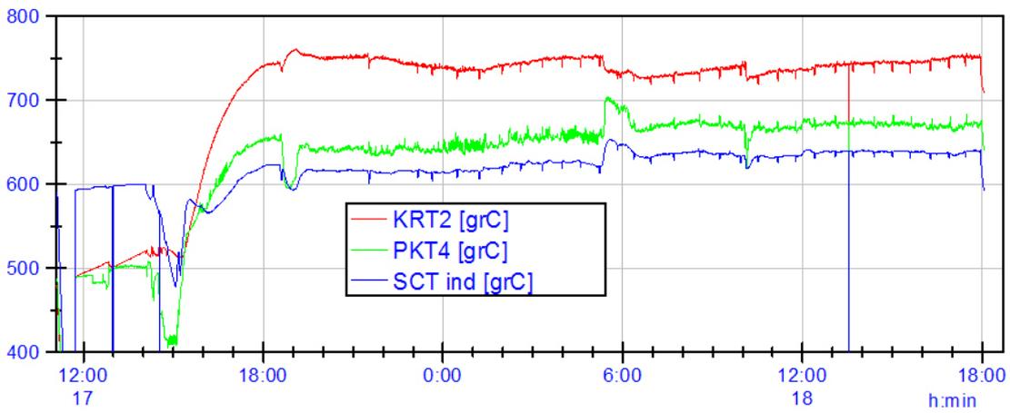
Figure 2.16 Important process temperatures from 100 kW<sub>th</sub> LT-CFB test no. 6
