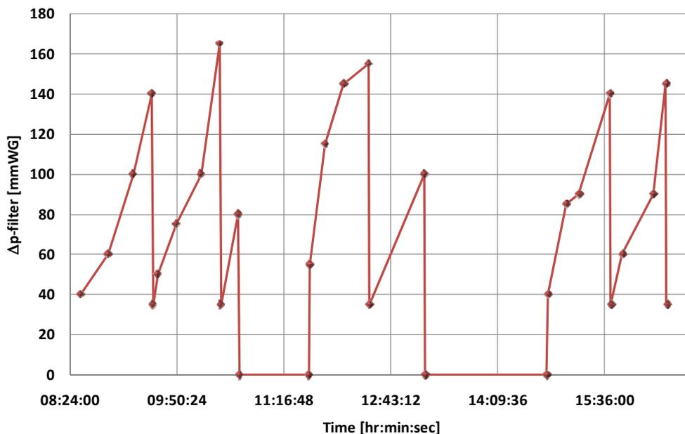
Figure 4.16 *Measurement of pressure drop across back house filter on September 24<sup>th</sup> 2009*
