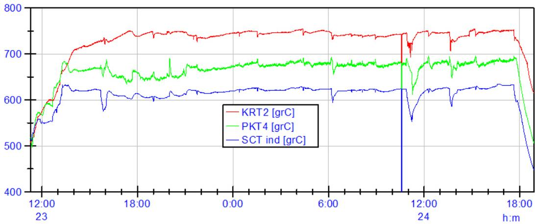
Figure 2.15 Important process temperatures from 100 kW<sub>th</sub> LT-CFB test no. 5
