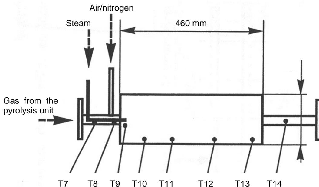
Figure 4.8 *Schematic drawing of the partial oxidation reactor*
