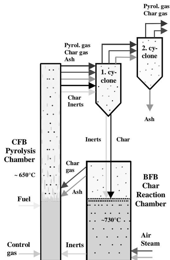
Figure 2.12 *LT-CFB flow diagram (simple version with a hot 2<sup>nd</sup> cyclone for gas cleaning)*
