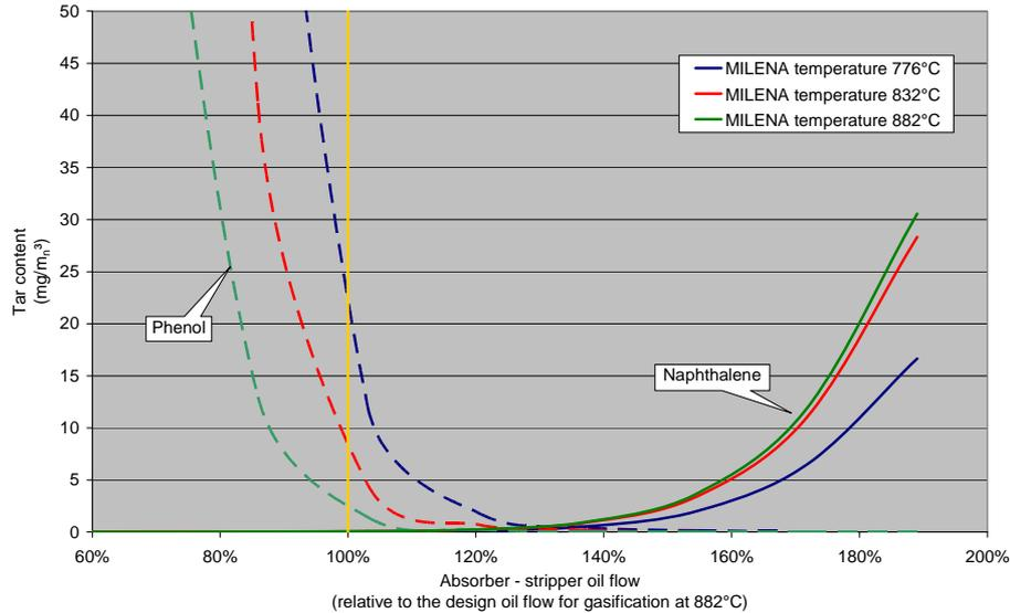
Figure 5.1 MILENA 10 MW<sub>th</sub> tar removal efficiency for different gasification temperatures
