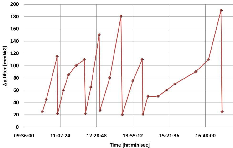
Figure 4.17 Measurement of pressure drop across back house filter on November 18<sup>th</sup> 2009
