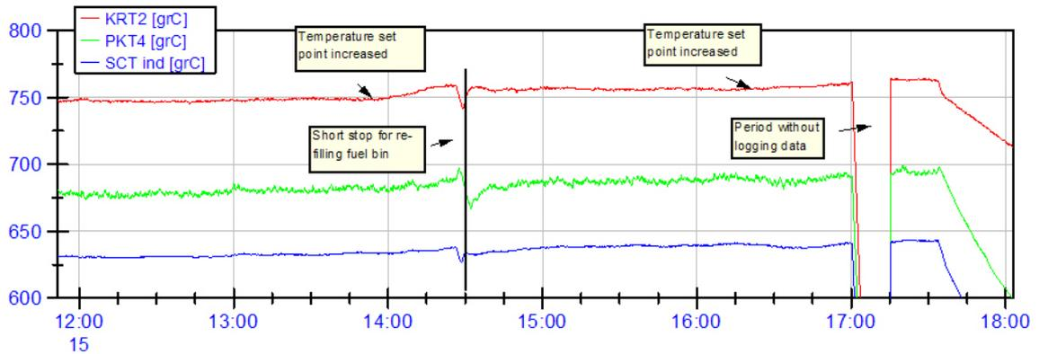
Figure 2.18 *Important process temperatures from last 6 hours of 100 kW<sub>th</sub> LT-CFB test no. 8*
