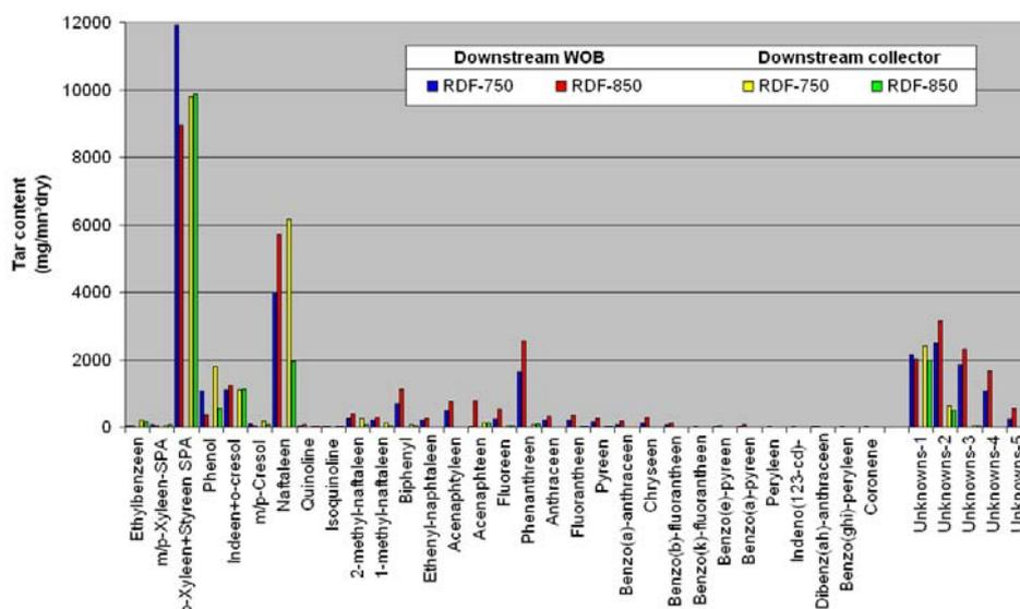
Figure 3.11 OLGA performance downstream RDF gasification at 750 & 850°C
