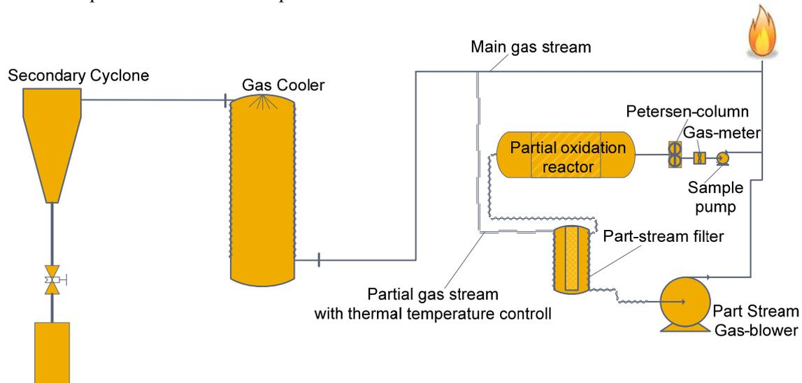
Figure 4.7 *Diagram of the gas cleaning set-up*
