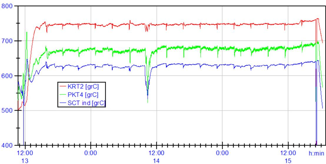
Figure 2.17 Important process temperatures from 100 kW<sub>th</sub> LT-CFB test no. 8
