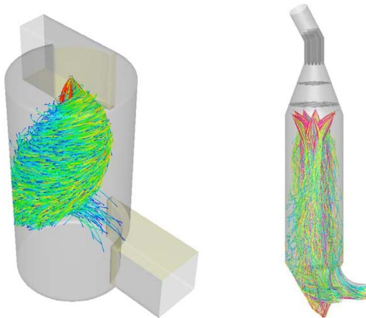
Figure 5.3 *Compact cooler design for gas coolers below 10 MW<sub>th</sub> (left) and cooling tower design for gas coolers above 10 MW<sub>th</sub> (right)*
