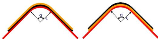
**Figure 5:** Test bench with a given shape (red) around which the module is to be bended in the convex way (left) and in the concave way (right):
