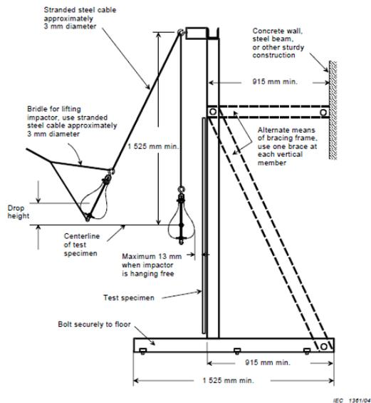
**Figure 2** Construction and test set-up module breakage test (IEC 61730)
