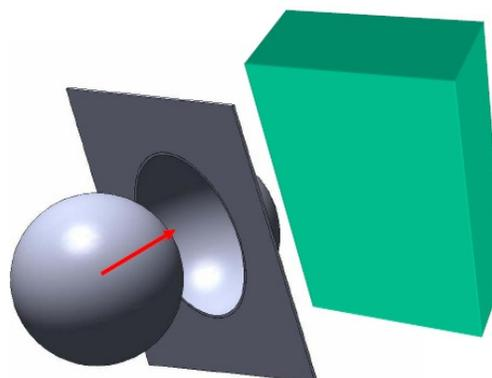
**Figure 6:** Schematic arrangement of a ball intrusion test
