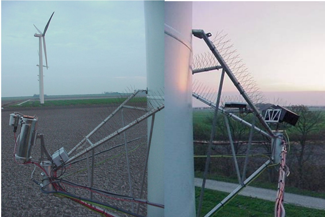
Figure 3a, b: Outdoor equipment of the WT-Bird prototype on tower of Nordex N80 turbine at EWTW
