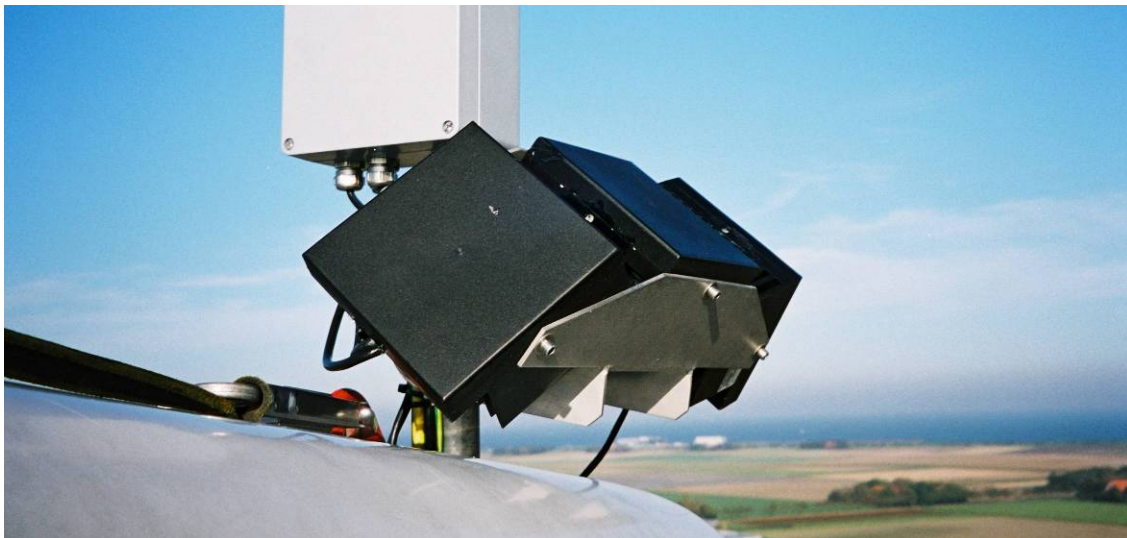
Figure 3c: Outdoor equipment of the WT-Bird prototype on nacelle of Nordex N80 turbine at EWTW
