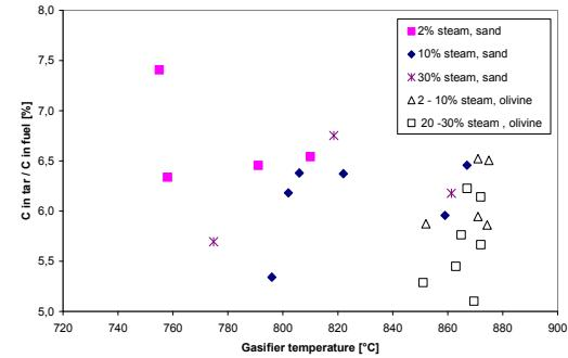
Figure 5: Effect of temperature on tar production
