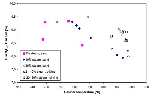
Figure 4: Effect of temperature on C<sub>2</sub>H<sub>4</sub> production
