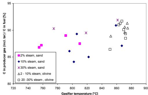
**Figure 6:** Effect of temperature on carbon conversion
