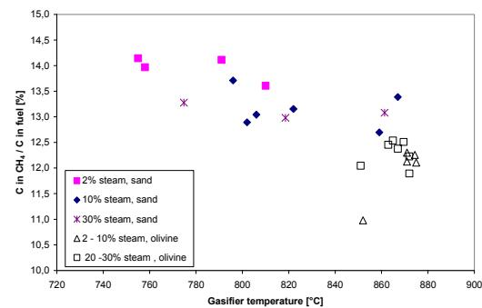
Figure 3: Effect of temperature on CH<sub>4</sub> production
