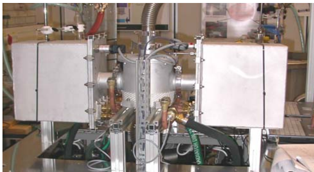
Figure 3.3 Picture of the 'thermal compressor' section of the adsorption cooling prototype system
