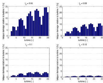
Figure 9: *Relative fatigue damage (turbine 1 = reference) of the 25 turbines for different values of ambient turbulence intensity.*
