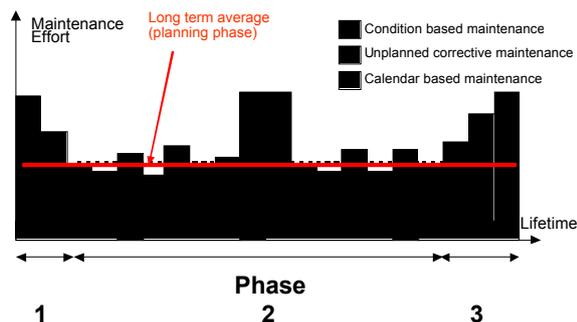
Figure 1: Schematic overview of the maintenance effort over the lifetime of an offshore wind farm.
