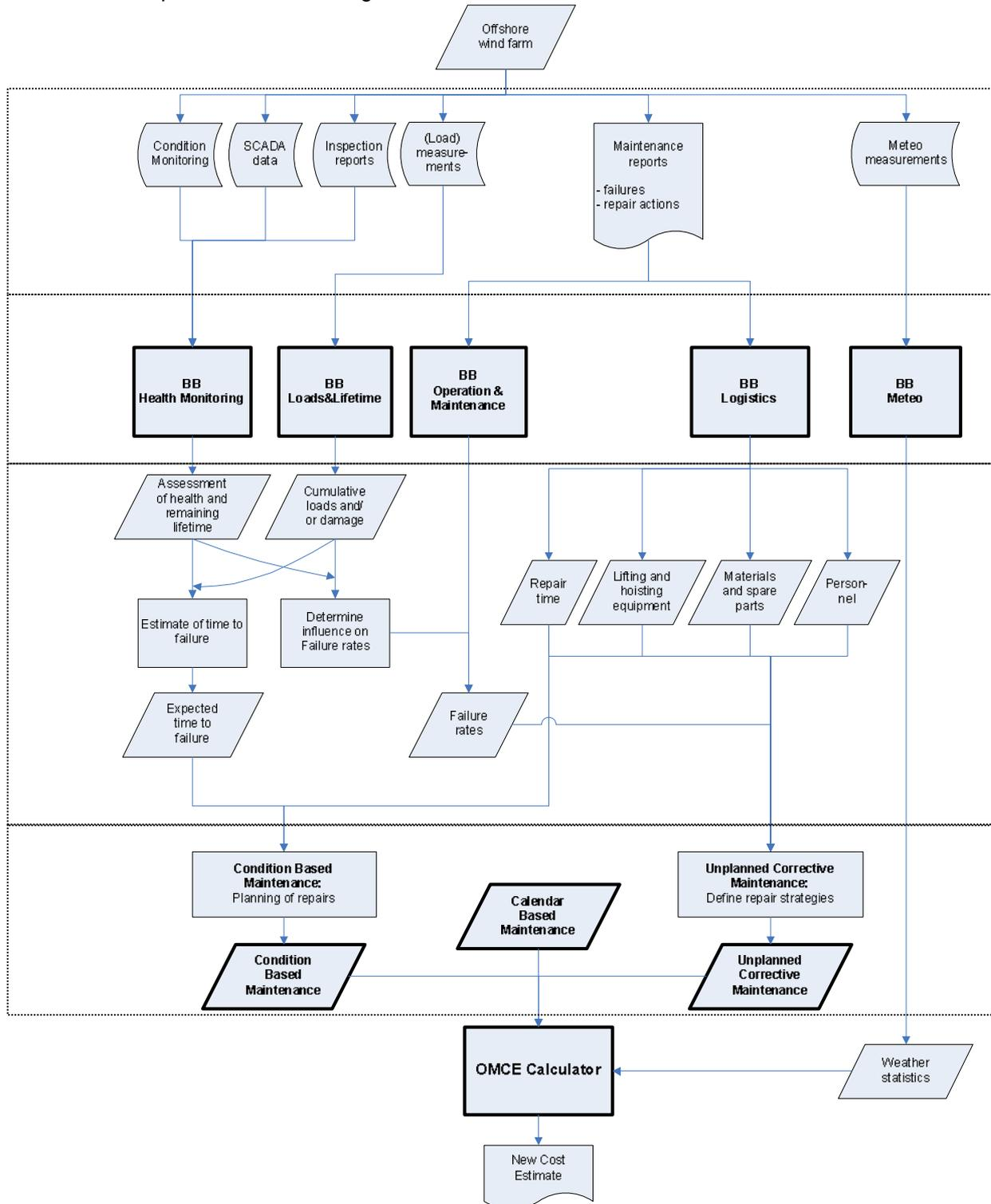
Figure 3: Structure for the O&M Cost Estimator
