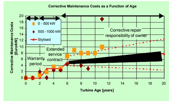
Figure 2: Development of the costs for unplanned corrective maintenance in the different stages of the lifetime [3].
