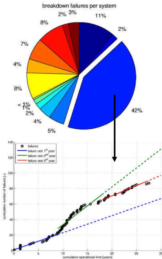
Figure 5: In the upper figure, the percentage of failures per component is presented. For the largest contribution, the cumulative number of failures as function of cumulative operational time is presented in the lower figure.
