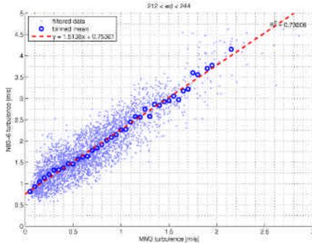
Figure 8: Correlation between turbulence measured at the nacelle of a N80 turbine and turbulence measured at a meteorological mast
