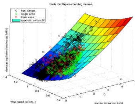
Figure 7: Correlation between turbulence, wind speed deficit and equivalent flapwise load ranges (using  $m = 7$ ), measured at ECN wind turbine test site Wieringermeer
