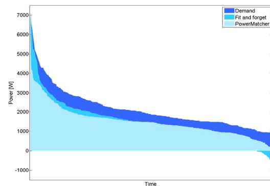
Figure 5: Load duration curve of the substation demand pattern without  $\mu$ -CHP, with  $\mu$ -CHP in a fit and forget strategy, and with PowerMatcher coordinated  $\mu$ -CHP.
