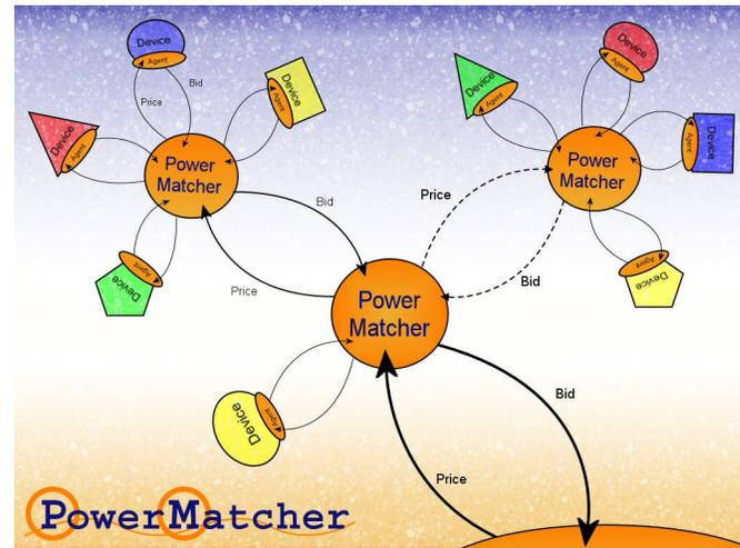
Figure 2: The PowerMatcher architecture; coming from a hierarchy based mechanism, growing towards a more organic, network of networks.
