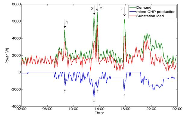
Figure 4: Time series of the substation demand pattern (green), the total  $\mu$ -CHP production (blue) and the net substation load (red) for 5  $\mu$ -CHPs with PowerMatcher coordination.
