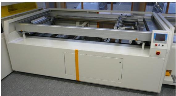
**Figure 5:** Interconnection, deposition of conductive adhesive
