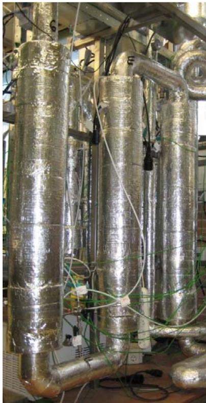
Figure 2.4 *Set of three vessels with absorbents for removal of Cl and S from gas.*
