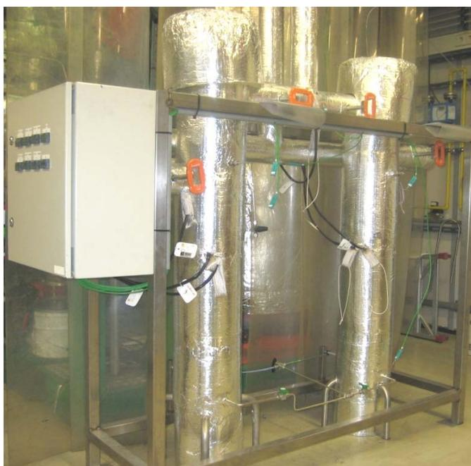
Figure 2.3 Set of hot gas filters with temperature control unit (left). The orange handles allow opening and closing of high-temperature valves for switching between filters.
