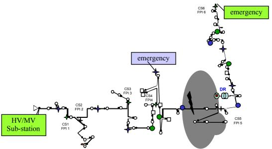
Figure 6-7 Fault localization principles step 4: elementary faulty area isolated manually
