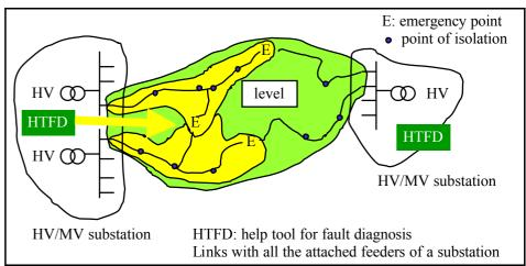
Figure 3-5 distribution network operated in open loop scheme
