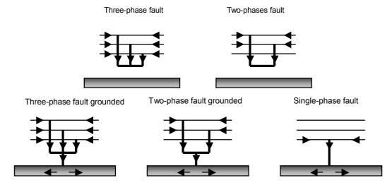
Figure 2-1 Fault types
