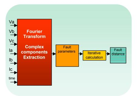
Figure 6-3 Fault distance evaluation principle
