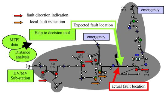
Figure 6-5 Fault localization principles step 2: the fault is cleared and investigated
