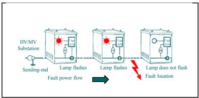
Figure 4-1 Non-directional FPI principle
