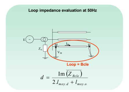
Figure 6-2 Loop impedance used for fault distance evaluation
