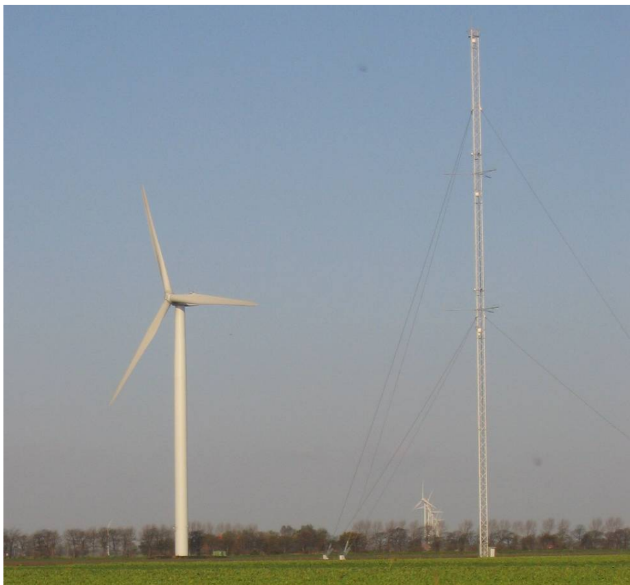
Figure 2.6: Nordex N80 turbine nr. 6 with meteo mast nr. 3 at ECN Windturbine Test site Wieringermeer (EWTW)
