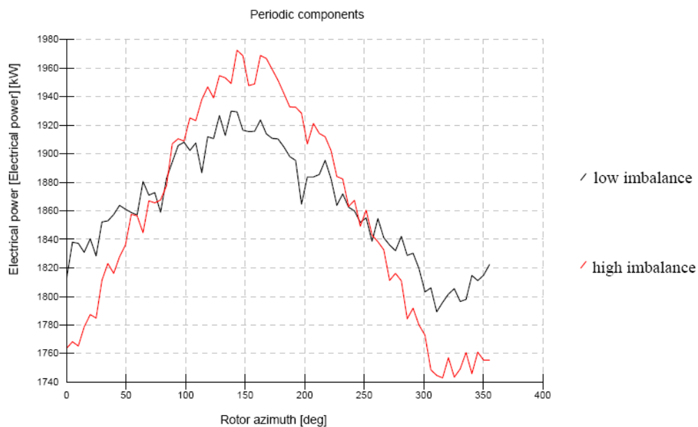
Figure 2.25: Fault modeling: rotor mass imbalance, 12 m/s, electrical power
