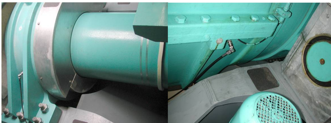
Figure 2.4: Vibration sensors of Prüftechnik system mounted on main bearing and 2 nd gearbox stage
