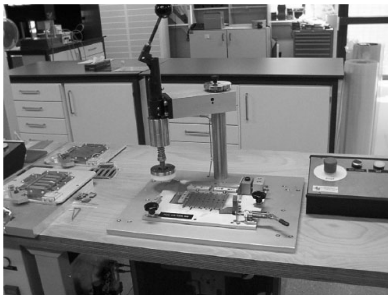
Figure 3. Pre-lamination unit for fixation of the polymer hot-melt to the TCO glass plates
