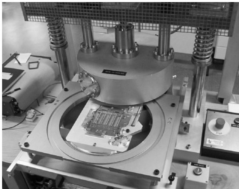
Figure 5. Vacuum laminator press for lamination of photoelectrode and glass counter-electrode with a polymer hot-melt
