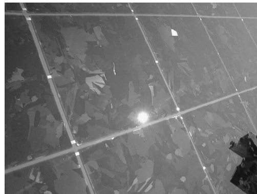
Fig. 5: Front surface of a 36 cells EWT module showing the homogeneous appearance without front metallisation.
