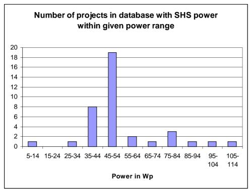
Figure 4.1 Distribution of module power for the solar home systems in the database
