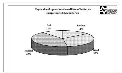
Figure 4.4: The physical and operational condition of a sample of 2,026 batteries from 1,743 solar home systems in Mexico (preliminary results) [Huacuz et al, 2000].
