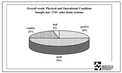
Figure 4.2: The physical and operational condition of 1,743 solar home systems in Mexico (preliminary results) [Huacuz et al, 2000].
