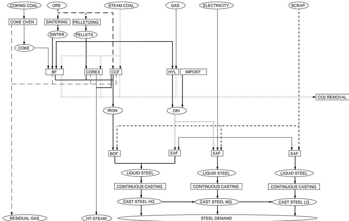
Figure 10.1 Steel model structure (HQ= High quality steel; MQ = medium quality steel; LQ = Low quality steel)
