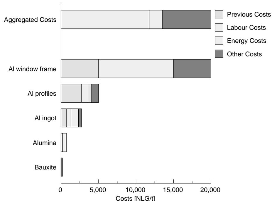
Figure 5.1 *Cost structure in the aluminium chain*
