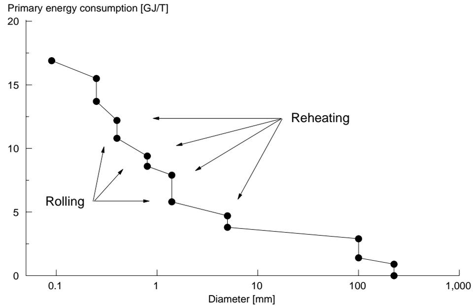
Figure 6.3 Energy consumption for conventional rolling and drawing from ingot to wire (Stainless steel 2333) [82]
