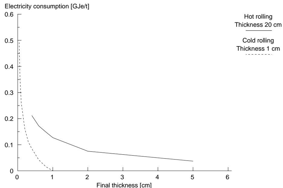
Figure 6.2 *Electricity requirement for rolling as function of the sheet product thickness [79]*
