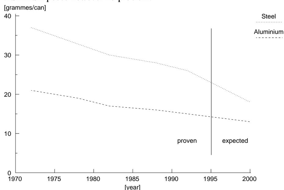
Figure 3.7 *The downward trend in steel and aluminium beverage can weight in the United States [50]*
